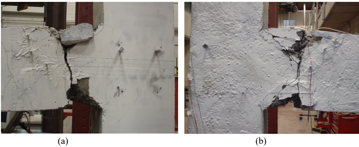
Fig. 12 – Crack pattern of specimens after being subjected to cycles up to 72 mm (2.83 in): (a) front face of JBC-3; and (b) rear face of JBC-3.
